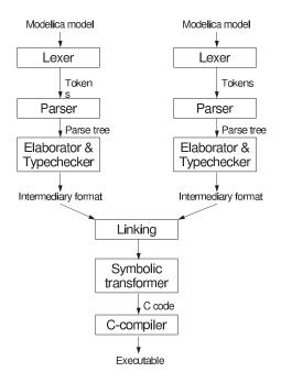
Figure 5: Separate compilation in Modelica.
