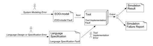
Figure 2.1: Relations between possible errors and faults in a M&S-environment.
