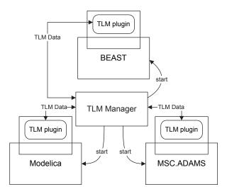
Figure 5: SKF's TLM system framework.
