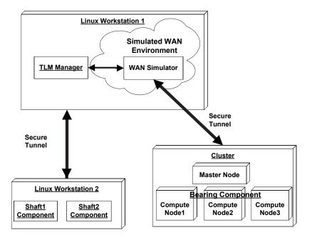
Figure 6: The deployment structure of the static structure of the system.
