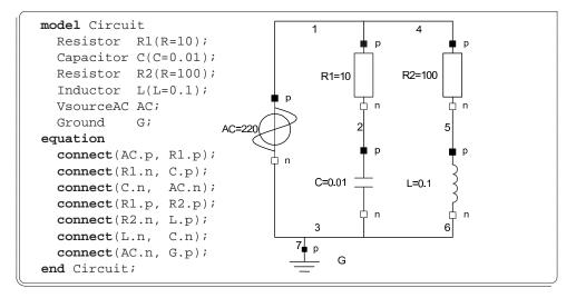
Figure 1.1: Modelica model of an electrical circuit.
