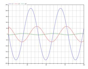
**Figure 2:** Plot of simulation result of the simple circuit. The largest curve shows the voltage source, the second largest the voltage drop over the inductor, and the smallest one the voltage drop over the capacitor.
