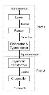
Figure 2: The structure of a Modelica compiler.
