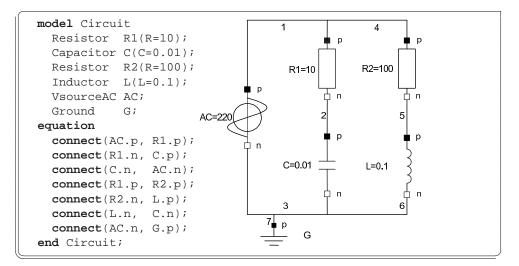
Figure 1: Modelica model of an electrical circuit.
