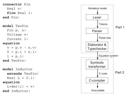
Figure 1.2: Source code of the Inductor model and its base class TwoPin.
