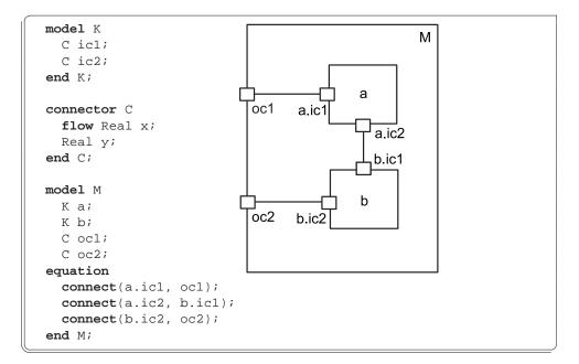
**Figure 8:** Model M with inside connectors (e.g. a.ic1 and b.ic2) and outside connectors (oc1 and oc2).
